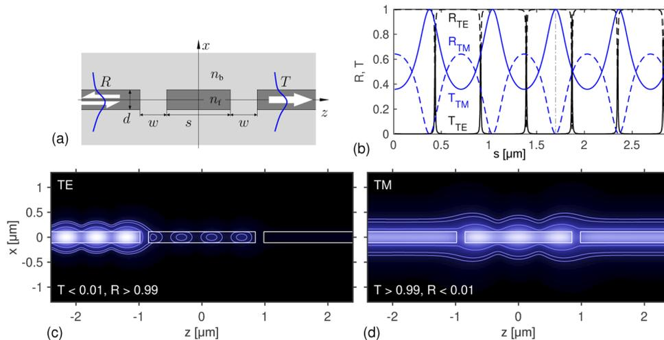
**Fig. 9.** Concept for a polarization beam splitter (a), based on two trenches of width  $w$  at a distance  $s$ ; all other parameters are as given for Fig. 1. (b) Reflectance  $R$  (dashed) and transmittance  $T$  (continuous) versus the distance  $s$ , for TE and TM excitation at  $\theta = 55^\circ$ , for  $w = 133 \text{ nm}$ . (c, d) energy-density  $u$  on the  $x$ - $z$ -plane for the splitter with separation  $s = 1.698 \mu\text{m}$ , for TE (c) and TM input (d).
