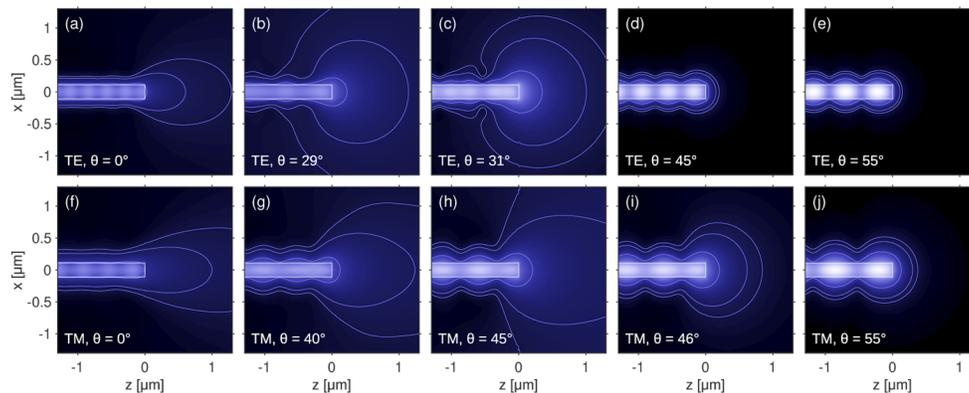
**Fig. 3.** Oblique incidence of semi-guided waves at a slab waveguide facet; energy density  $u$  of the optical electromagnetic field on a  $x$ - $z$ -plane perpendicular to the facet, for TE (top row) and TM input (bottom row) at angle  $\theta$ ; contour lines at 5%, 1%, and 0.5% of the maximum level, with a uniform color scale for all panels.
