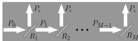
**Fig. 8.** Concept for a  $1 \times M$ -equal-power divider. A sequence of trenches, each with potentially different width, are arranged along the axis of an incoming semi-guided wave bundle with input power  $P_0$ . Each trench with reflectance  $R_j$  diverts the power  $P_c$  from its input  $P_{j-1}$  into one of the  $M$  output “channels”.
