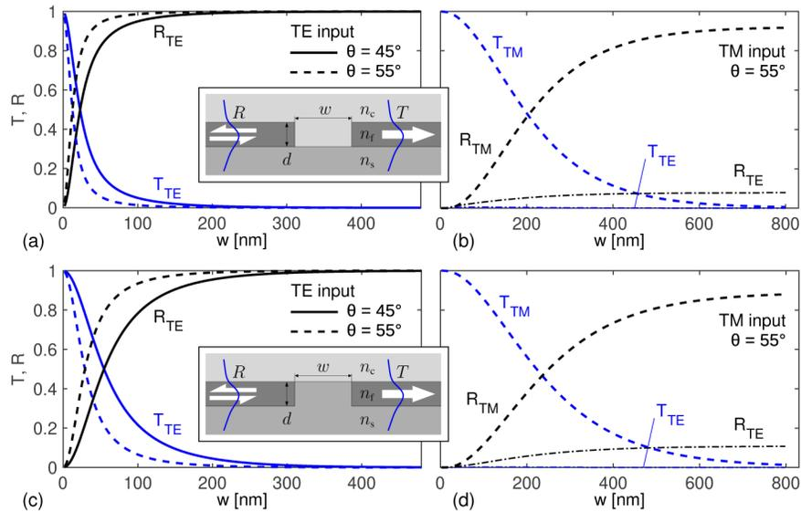
**Fig. 11.** Oblique incidence of semi-guided waves on trench structures with nonsymmetric layering, with refractive indices  $n_s : n_f : n_c = 1.45 : 3.45 : 1.0$  and air gap (a, b), and a filled trench (c, d). Reflectance  $R$  and transmittance  $T$  versus the trench width  $w$ , curves for TE (a, c) and TM excitation (b, d), at angles  $\theta = 45^\circ$  (continuous) and  $\theta = 55^\circ$  (dashed, dash-dotted).
