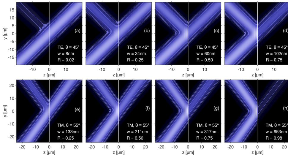
**Fig. 7.** Power dividers of width  $w$ , excitation by TE- (a-d) or TM-polarized (e-h) semi-guided Gaussian wave bundles of cross-sectional width  $W_b = 7 \mu\text{m}$  at angle  $\theta$  leads to a reflectance  $R$  and transmittance  $T = 1 - R$ ; energy density  $u$  of the optical electromagnetic field, contour lines at 5%, 1%, and 0.5% of the maximum level, with a uniform color scale for all panels.
